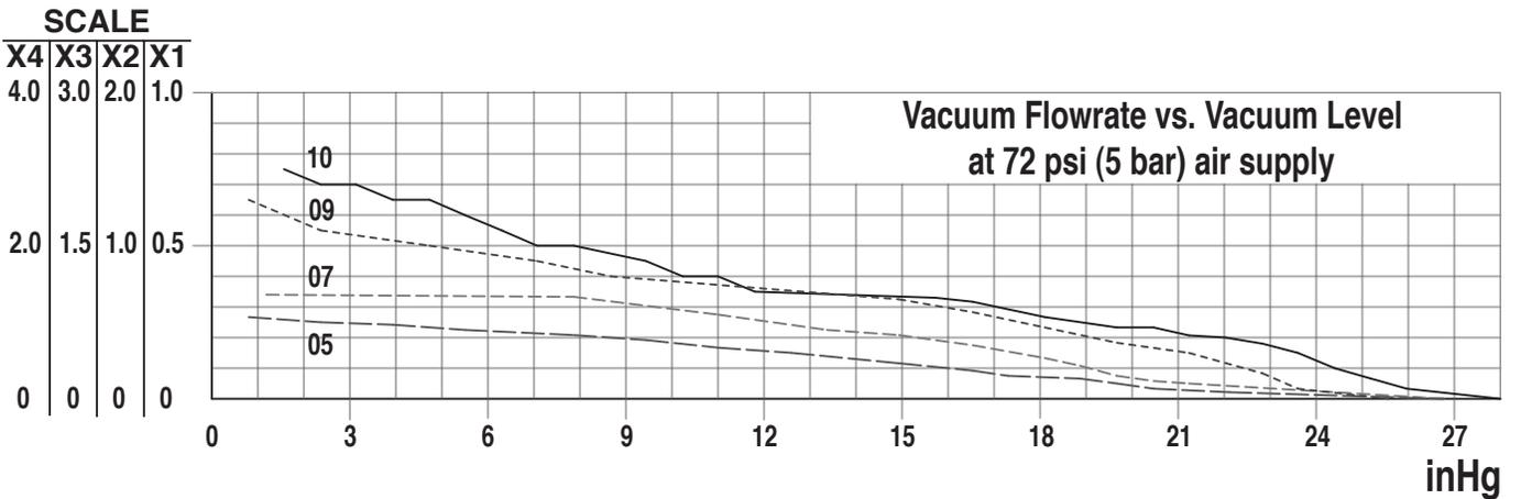
All performance data presented is a representation of production pumps but is not a guarantee due to variations in local barometric pressure and of mass produced components.
